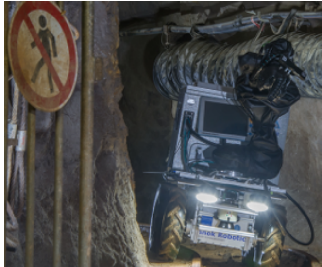
Fig. 1. Research robot returning from its exploration of an restricted area within a silver mine. Under difficult underground environmental conditions, this robot focuses on endurance and autonomy.
